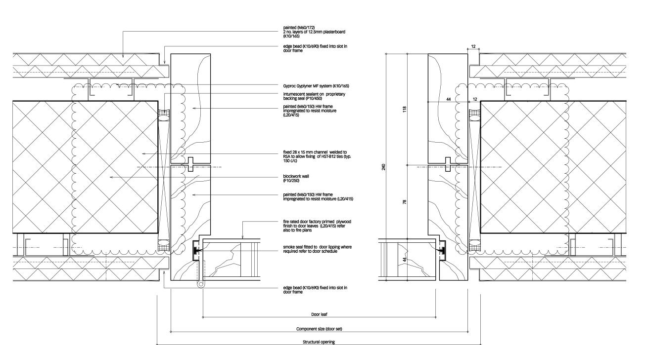
1) dry lined blockwork wall jamb detail
