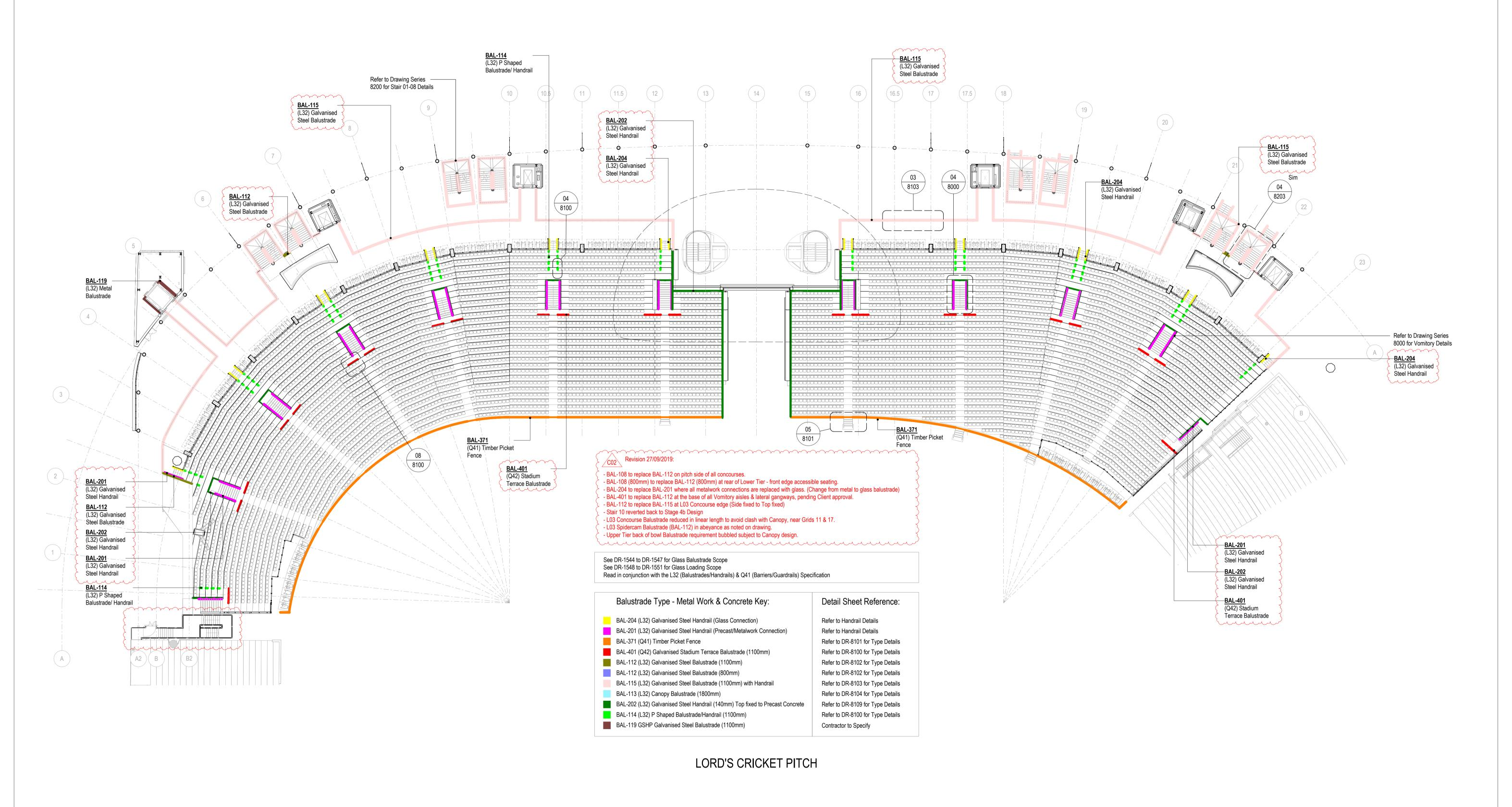
01 Level 01 Plan - Metalwork & Concrete Balustrade Scope
